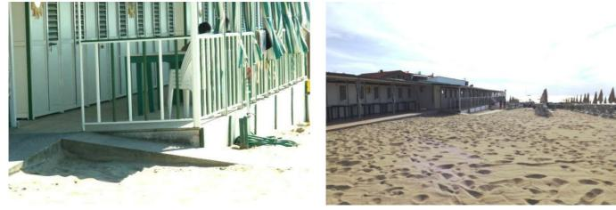
There are n. 1 toilets accessible / usable by people with reduced mobility. The toilets are accessible by ramp: length. 70 cm, width. > 100 cm, gradient 10%. The useful width of the bathroom door is 92 cm.
