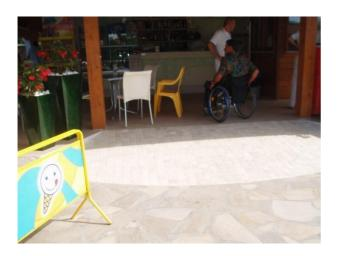
The restaurant bar is accessible by ramp: length. 168 cm, width. > 100 cm, gradient 10%. The useful width of the door / gate input is greater than 90 cm.
